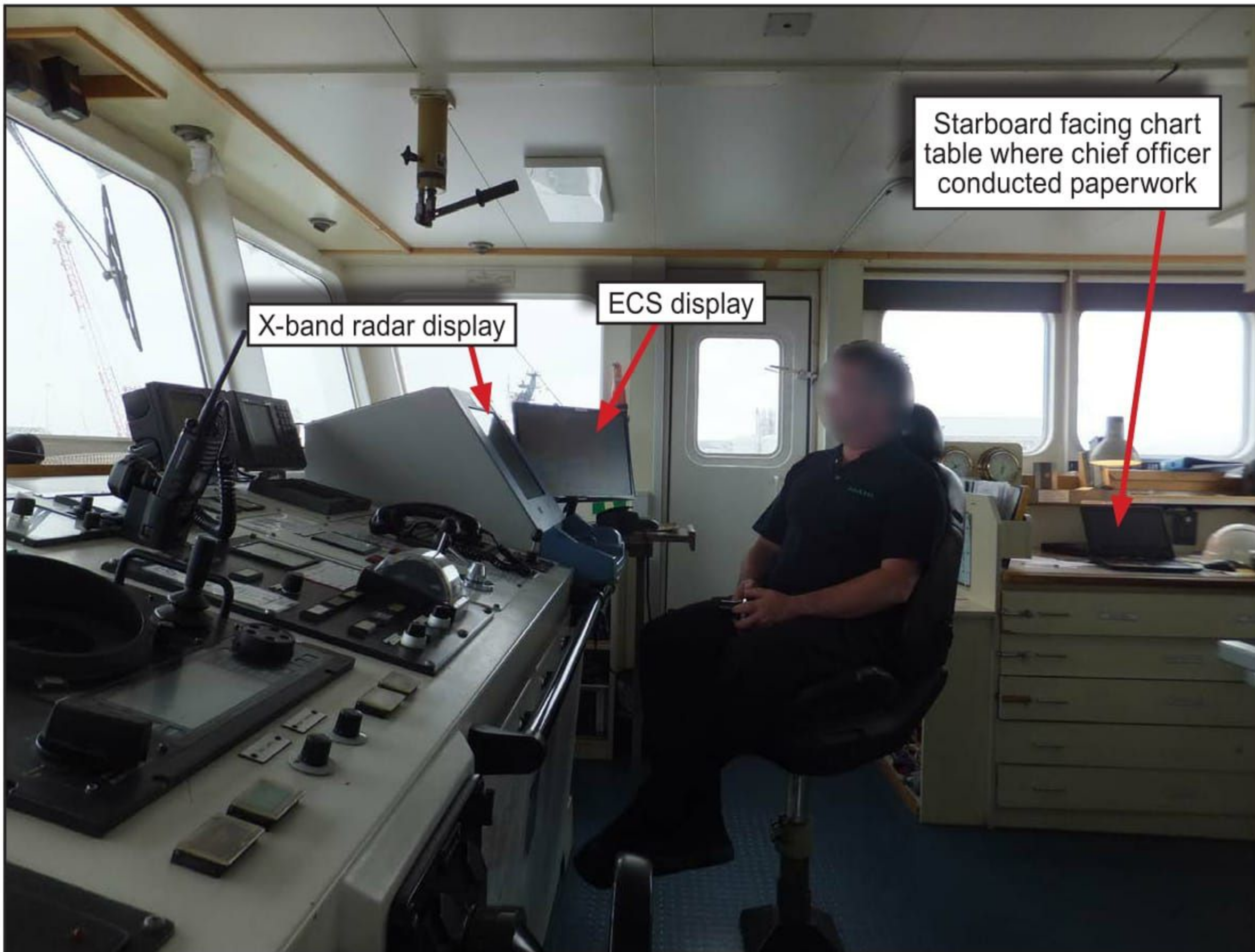
Figure 3: Reconstruction of the chief officer of Daroja sitting in the chair on the starboard side of the bridge prior to collision
