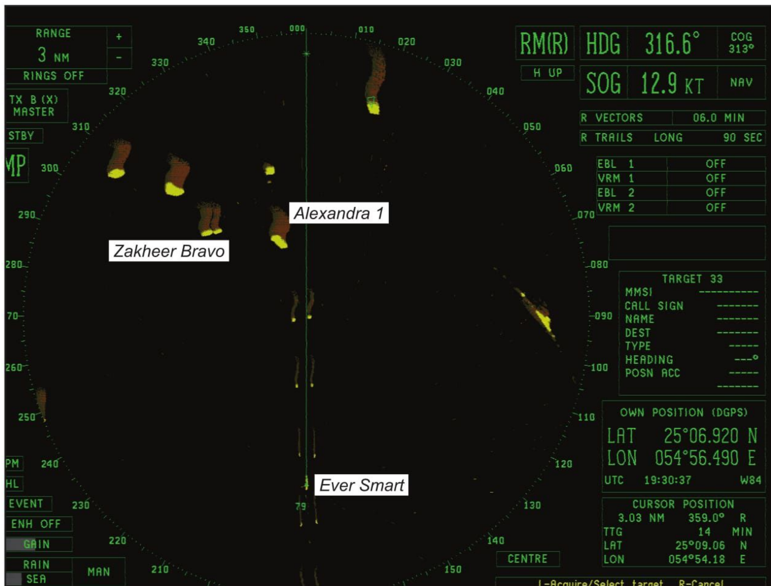
Figure 4: Ever Smart – port radar display at 2331
