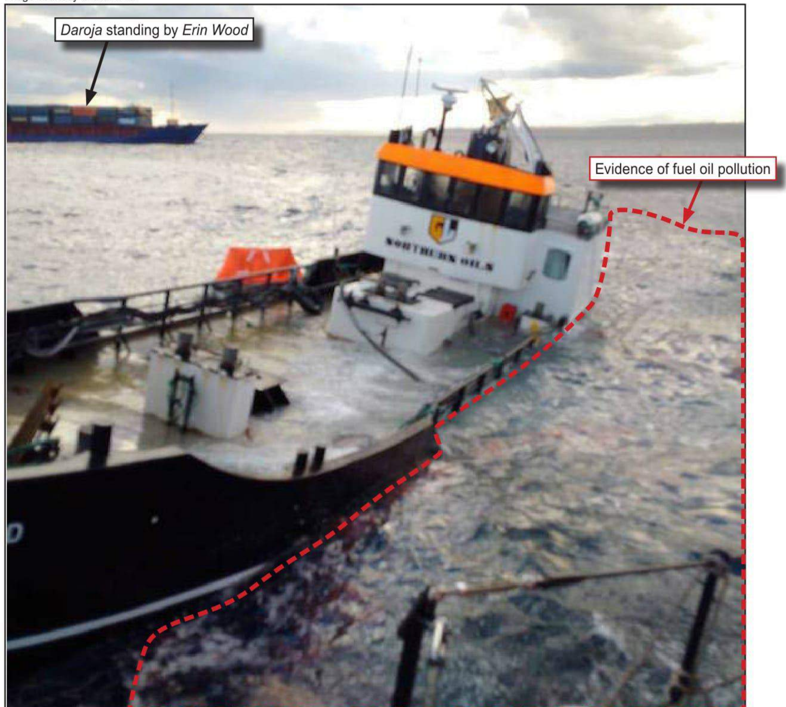
Figure 6: Erin Wood after the collision as seen from the Peterhead lifeboat, including evidence of fuel cargo pollution
