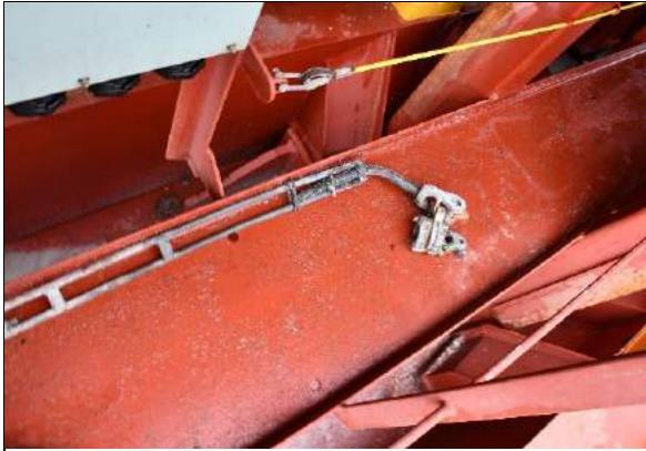
Figure 13: Bent turnbuckle (Source: German Waterway Police)
