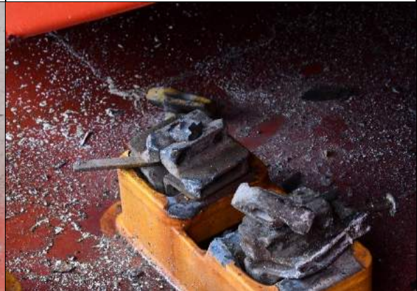
Figure 16: Broken turnbuckle (Source: German Waterway Police)
