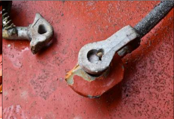
Figure 14: Broken mount from lashing bridge (Source: German Waterway Police)
