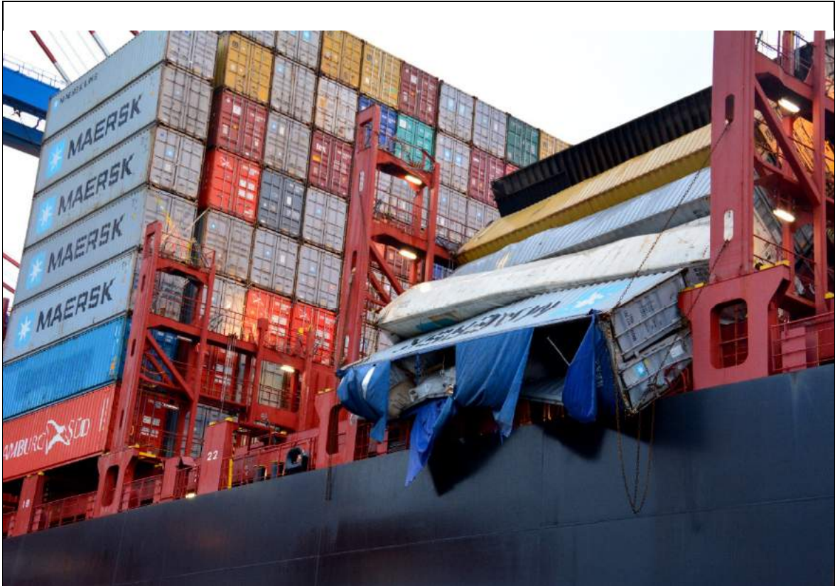
Figure 5: Container with bags with polystyrene balls hanging over the side. (Source: DSB)
