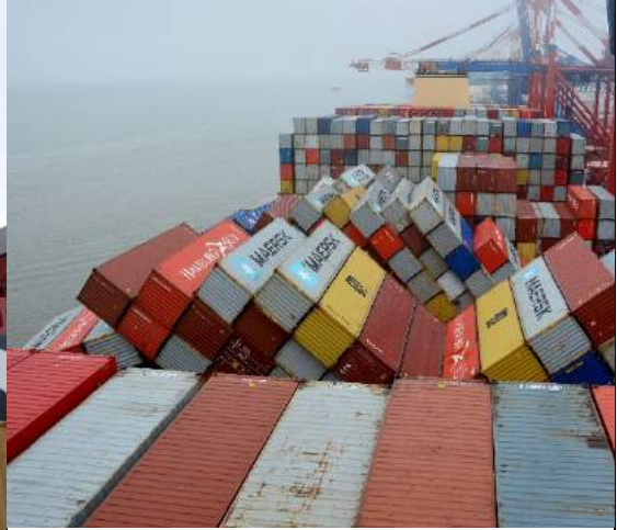
Figure 8: Collapsed containers in bay 26. (Source: BSU)
